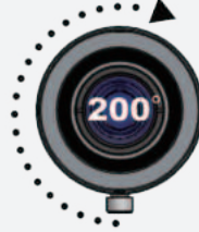
Existing Lens Focus ring rotation angle: 200°
